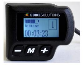
Press MODE briefly to display the average speed "AVG" since the last time the display was switched on instead of "Ridtime":
