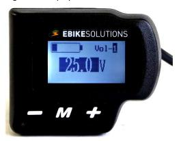
Once you have selected the appropriate voltage value (voltage values between 20.0 V and 60.0 V are possible), briefly press **MODE** to confirm: The display changes to "Vol-2", a bar display with 2 battery segments and a dark volt number.
