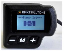
In addition to 3, 5, 7 or 9 support levels, you can select whether level "0" should also be available or not. In level "0", data is shown on the display, but there is no support from the PAS sensor when you pedal.
