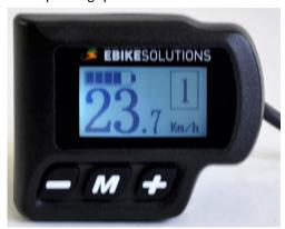
Press MODE briefly to display the total distance travelled since the last reset of the short distance counter "TRIP" instead of the current speed:
