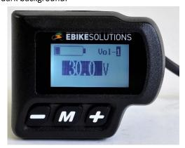
Use UP or DOWN to set the voltage value up to which 1 battery segment should still be visible in the display. If the battery voltage falls below the value listed under "Vol-1", the empty frame of the battery display flashes in the display and the motor is switched off.
