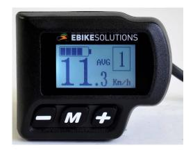
Press MODE briefly to show the maximum speed "MAX" instead of "AVG" since the last time the display was switched on:
