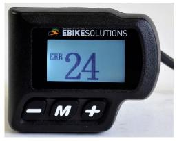
The display will not return to normal until the fault has been rectified. Until then, the system must no longer be used. If you cannot correct the fault yourself, please contact our customer service. You will find the contact information at the end of these operating instructions. Do not attempt to open or improperly manipulate the conversion kit or its components.
