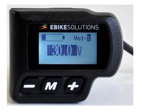
EBS delivers the display with a "VOL-1" value equal to "25.0 V". You should also store this value again after resetting the display to the factory settings of the display manufacturer:
