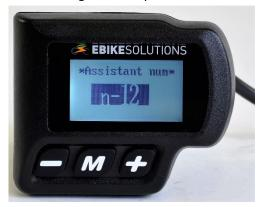
If the magnetic disc of your EBS conversion set has 12 magnets, please leave it at the factory setting "n-12" and do not make any changes here. Then briefly press MODE to confirm: The display briefly shows "OK!" and then jumps back to "Specific Set".
